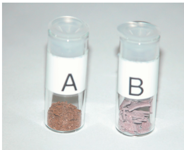
Figure 1. Photograph showing solution-precipitated blends of (A) 0.6 mol % poly(ethylene oxide)/ C_{60} and (B) 1.4 mol % polystyrene/ C_{60} .
